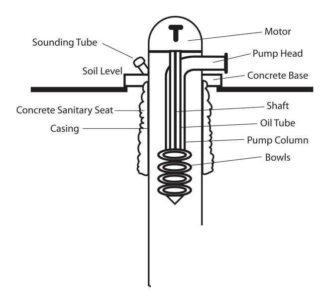
**Well cap or seal:** The well should be completely sealed against surface water, insects or other foreign matter. Look for holes, missing plugs and leaking water (artesian flow). If water is coming out, then contaminants can seep into the well. Replace any missing plugs and seal any openings, gaps or cracks.
