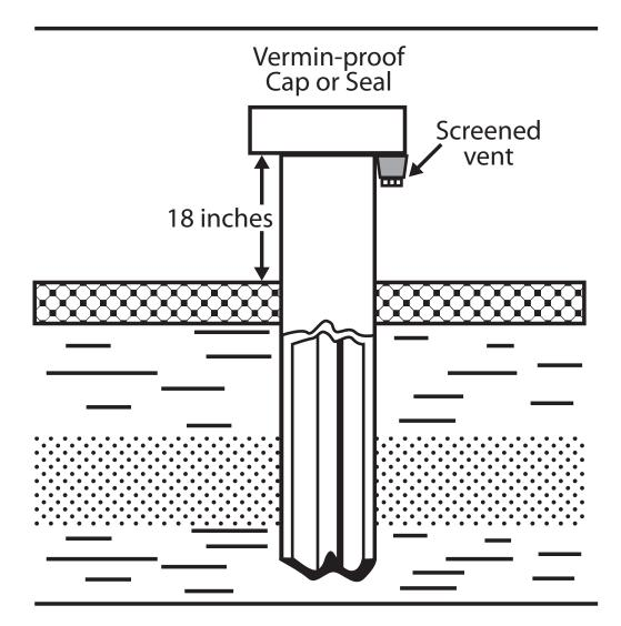
**Well vent:** Check the cleanliness and integrity of the well vent screen. Look for tears or holes. Vents must be covered with a screen. Replaced damaged vent screens.
